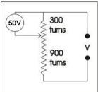
**Explanation.** This is a standard potentiometer. It splits the voltage by the same ratio as the number of turns. So 50V is 300/1200ths of the source voltage (50 = 3/12V). Transpose for V.
