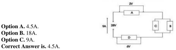
**Explanation.** You need to know what the ohmic value of resistor C is to know the current through it, or at least the relative value of C compared to D - as the 9A current splits through C and D. It is 9A/2 (4.5A) only if C and D are the same. Besides, it cannot ever be 9A or 18A.
